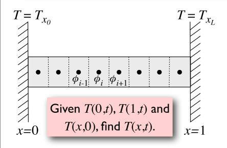
$$\frac{\partial T}{\partial t} = \alpha \frac{\partial^2 T}{\partial x^2}$$
