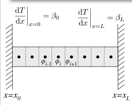
$$\frac{\partial T}{\partial t} = \alpha \frac{\partial^2 T}{\partial x^2}$$
