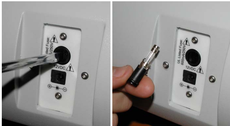
Figure 18: Replacing a Fuse
