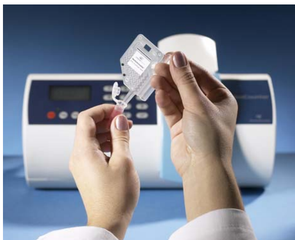
Figure 9: Loading the Cassette
