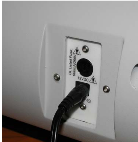
Figure 4: Power Supply Cord Connection (Rear Panel)
