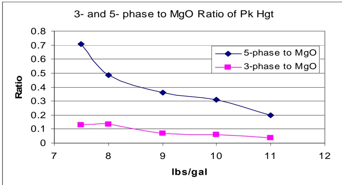
**Figure 5. Plot of the ratio of 24-hour x-ray peak heights corresponding to the 5-phase to MgO ratio and the 3-phase to MgO ratio observed in Figure 3 are plotted as a function of the “impure”  $33.2 \pm 0.17\%$  MgCl<sub>2</sub> brine to MgO ratio.**
