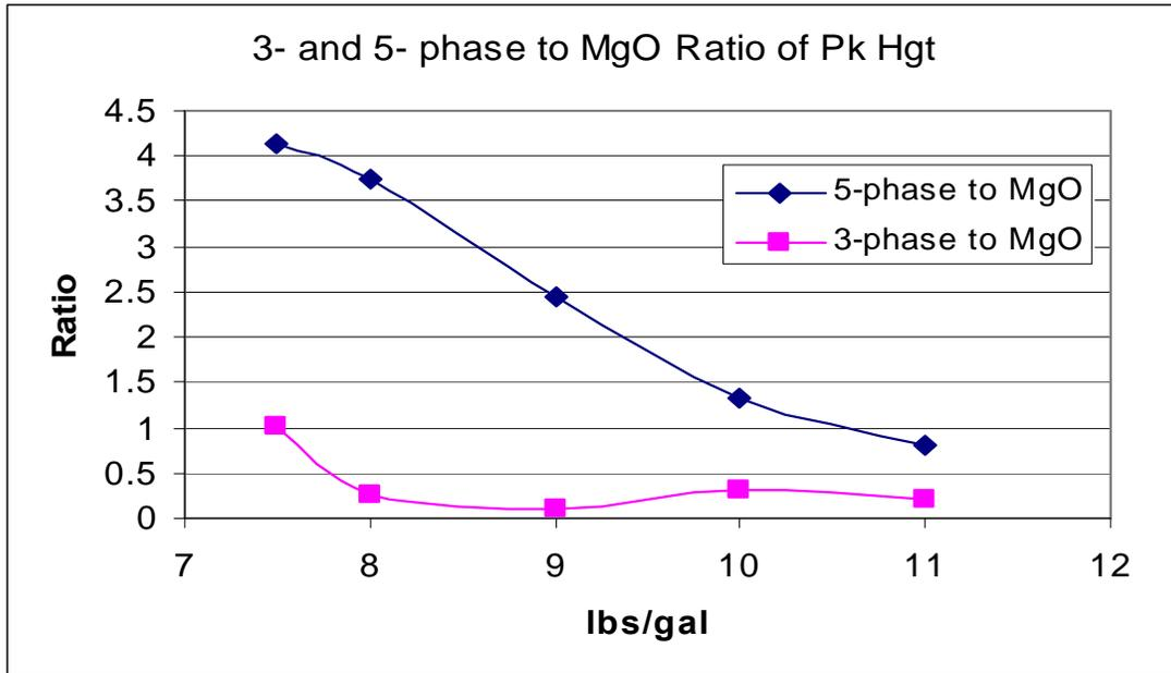
**Figure 12. Plot of the ratio of 24 hour x-ray peak heights corresponding to the 5-phase to MgO ratio and the 3-phase to MgO ratio observed in Figure 7 are plotted as a function of the “pure”  $28.9 \pm 0.15\%$   $MgCl_2$  brine to MgO ratio.**
