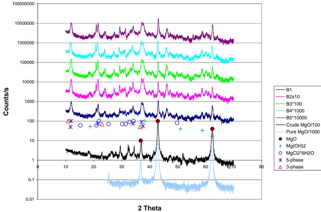
**Figure 7. X-ray diffraction analyses of cements allowed to set for 24 hrs. These B series cements were made with various MgO to “impure”  $28.9 \pm 0.15\%$   $MgCl_2$  by weight brine ratios given in Table 2. Data points indicate the location and intensity of peaks according to JCPDS-ICDD.**
