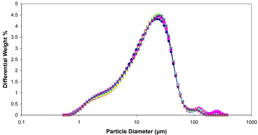
**Figure 2. Particle Size Distribution (Differential Volume vs. diameter) of Premier Chemicals MgO Powder using Beckmann Coulter LS230. The various traces correspond to replicate analysis taken at 1-minute interval. Some small amount of aggregation is observed with the latter samples.**
