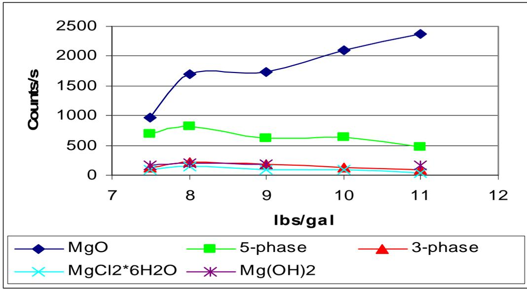
**Figure 4. Plot of 24 hour x-ray peak heights corresponding to MgO ( $2\theta=42.9^\circ$ ), 3-phase ( $2\theta=23^\circ$ ) and 5-phase ( $2\theta=11.9^\circ$ ) observed in Figure 3 are plotted as a function of the “impure”  $33.2 \pm 0.17\%$  MgCl<sub>2</sub> brine to MgO ratio.**
