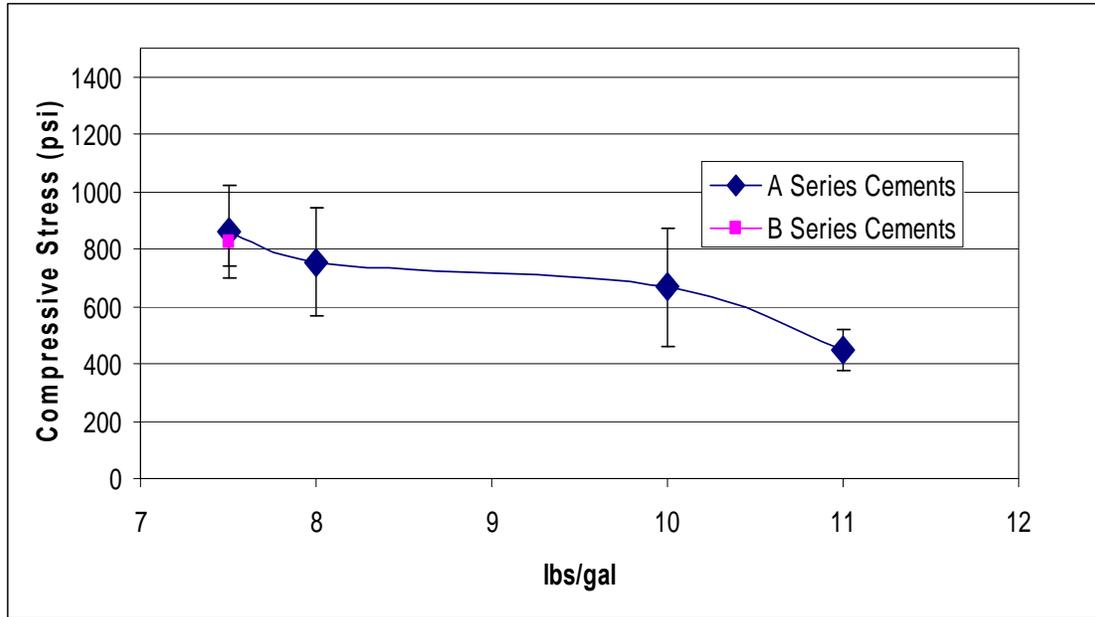
**Figure 16. Compressive Strength of Cements as a function of MgO to Brine ratio. These A series cements were made with “impure”  $33.2 \pm 0.17\%$  wgt  $MgCl_2$  by weight brine and the B series cement was made with “impure”  $28.9 \pm 0.15\%$  wgt  $MgCl_2$ . Error bars on the data points correspond to the standard deviation of 5 strength measurements.**
