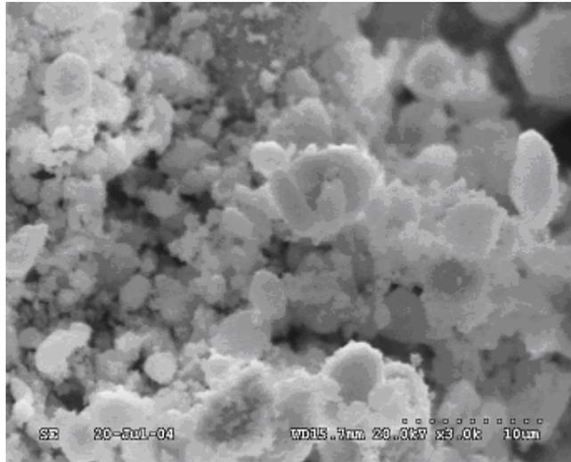
**Figure 1. SEM of Premier Chemicals MgO Powder at 3000x Magnification. Dotted Bar = 10 microns.**
