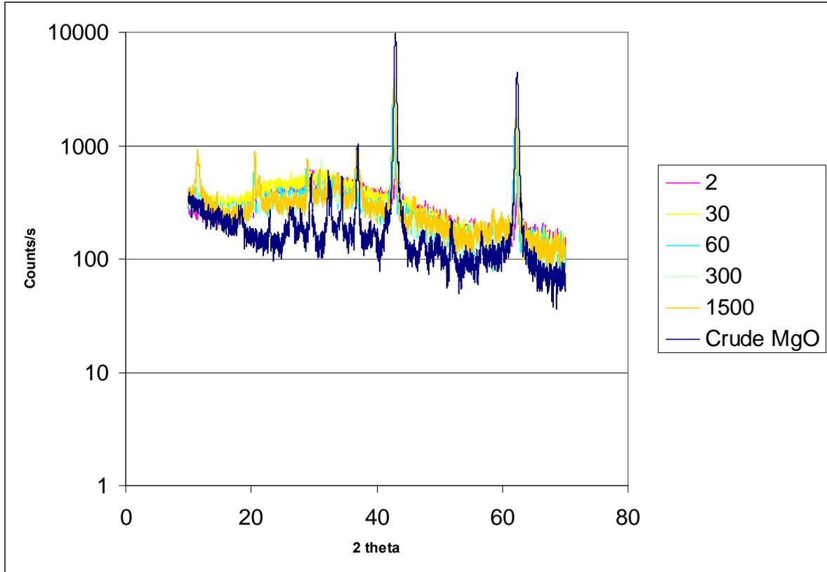
**Figure 20. x-ray spectra as a function of setting time in minutes for Cement A1 corresponding to 0.8987 kg/L (7.5 lbs/gal) “crude” MgO in 33.2±0.17% “impure” MgCl<sub>2</sub>.**
