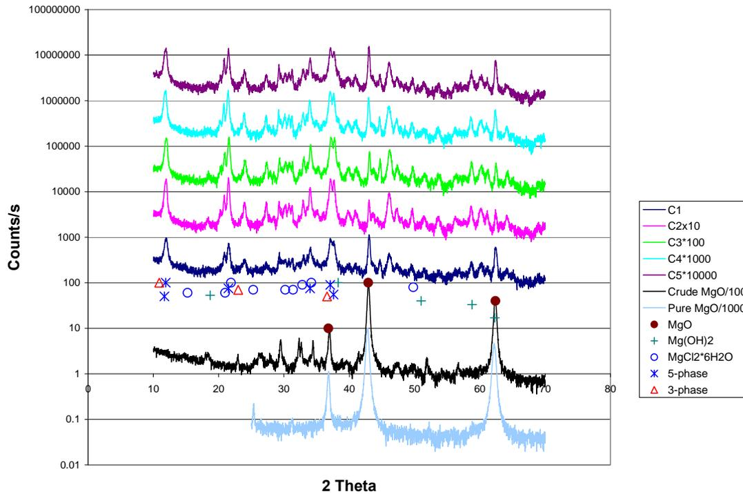
**Figure 10. X-ray Diffraction analyses of cements allowed to set for 24 hours. These C series cements were made with various MgO to “pure”  $28.9 \pm 0.15\%$   $\text{MgCl}_2$  by weight brine ratios given in Table 2. Data points indicate the location and intensity of peaks according to JCPDS-ICDD.**
