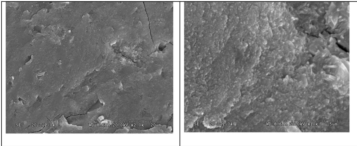
**Figure 6. Scanning Electron Micrograph of cement A1 at two magnifications; 2,000x (dotted bar = 20 microns) and 10,000x (dotted bar = 5 microns).**
