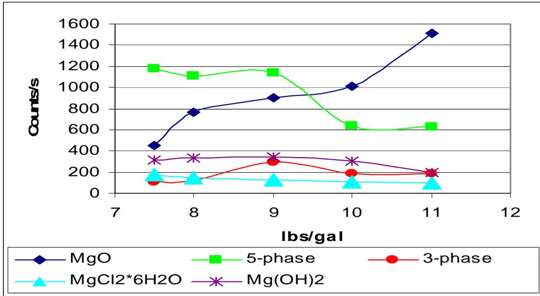
**Figure 8. 24 hour x-ray diffraction peak heights from Figure 7 versus MgO to cement ratio for impure  $28.9 \pm 0.15\%$  weight  $MgCl_2$  Brine and impure MgO.**
