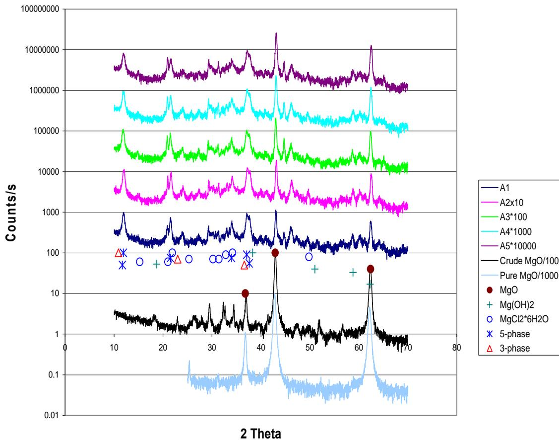
**Figure 3. X-ray diffraction analyses of cements allowed to set for 24 hours. These A series cements were made with various MgO to “impure”  $33.2 \pm 0.17\%$  MgCl<sub>2</sub> by weight brine ratios given in Table 2. Data points indicate the location and intensity of peaks according to JCPDS-ICDD.**
