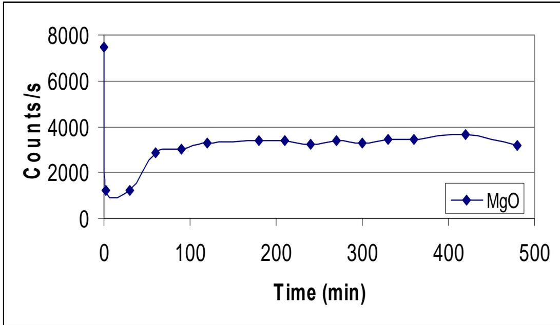
**Figure 19. X-ray peak height for MgO phase ( $2\theta = 42.9^\circ$ ) as a function of setting time for cement A1 0.8987 kg/L (7.5 lb/gal)  $33.2 \pm 0.17\%$  “impure”  $\text{MgCl}_2$  brine.**
