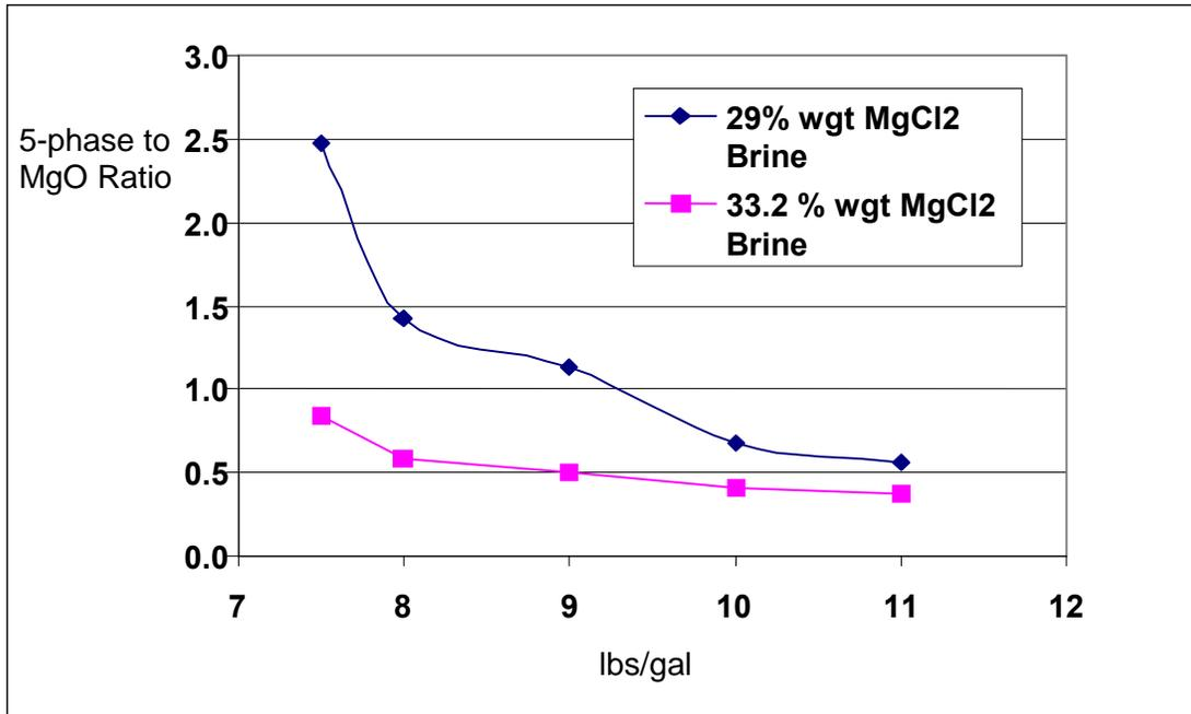
**Figure 13. Ratio of XRD peak heights for 5-phase to MgO in cements set for 24 hours with different ratios of MgO to brine. In both cases the brine is “impure” GSLM brine.**
