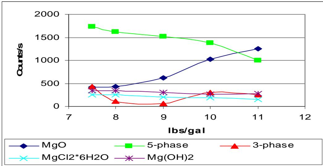
**Figure 11. 24 hour x-ray diffraction peak heights from Figure 7 versus MgO to cement ratio for “pure”  $28.9 \pm 0.15\%$  weight  $MgCl_2$  Brine and impure MgO.**
