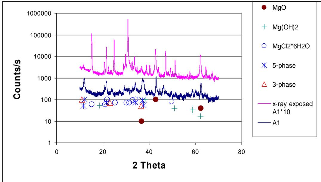
**Figure 17. 24 hour x-ray spectra of Cement A1 corresponding to 0.8987 kg “crude” MgO per liter (7.5 lb “crude” MgO per gal) of “impure” 33.2±0.17% MgCl<sub>2</sub> brine when sample is exposed to x-rays for 24 Hrs and when it is not exposed to x-rays.**
