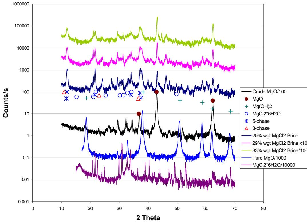
**Figure 14 X-ray diffraction data for cement samples allowed to set for 24 hours made with different Brine concentrations and 1.3181 kg/L (11 lbs MgO/gal).**
