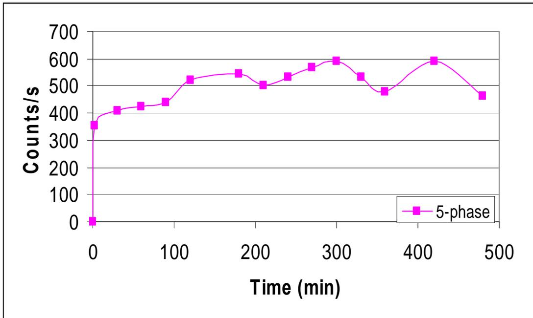
**Figure 18. X-ray peak height for 5-phase ( $2\theta = 11.9^\circ$ ) as a function of setting time.**
