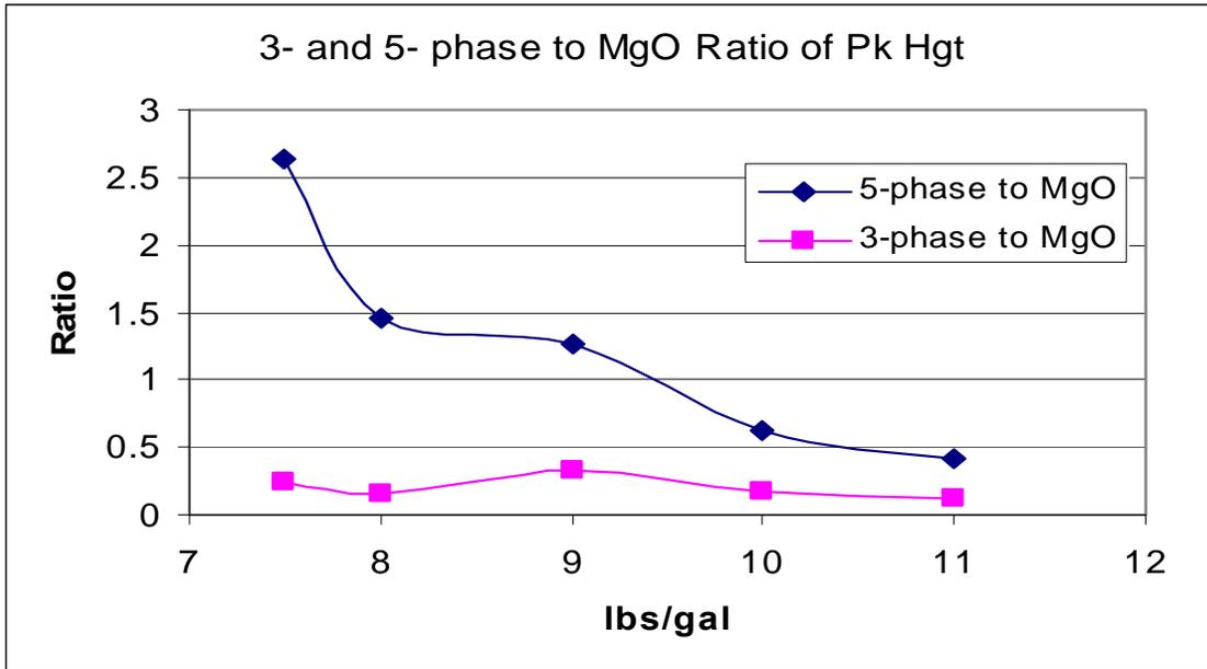
**Figure 9. Plot of the ratio of 24 hour x-ray peak heights corresponding to the 5-phase to MgO ratio and the 3-phase to MgO ratio observed in Figure 7 are plotted as a function of the “impure”  $28.9 \pm 0.15\%$   $\text{MgCl}_2$  brine to MgO ratio.**
