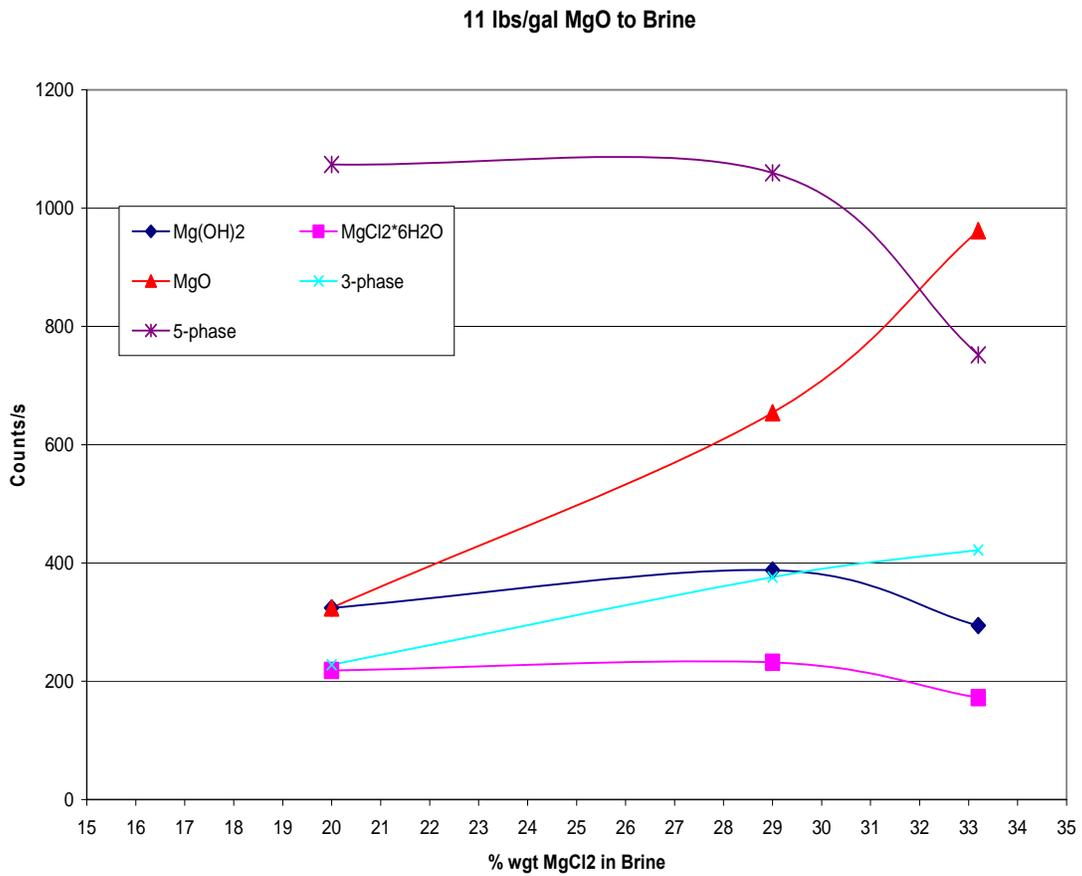
**Figure 15. 24 hour x-ray diffraction peak heights from Figure 14 versus “impure” MgCl<sub>2</sub> brine concentration from 20 to 33 % MgCl<sub>2</sub> for cements made with 1.3181 kg/L (11 lbs/gal) impure MgO to brine ratio.**
